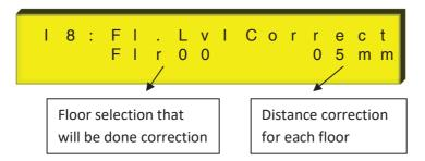
For each floor in shaft learning, at the situation of the car doesn't stop the floor level, it is used for accuracy correction. To enter the parameter, floor is selected with the arrow on left side by pressing ENTER button and by pressing again, distance correction is done as (-) or (+) value with arrow on the right side. Distances are indicated one by one or by using "All" option in the left side of parameter, the same correction for all floors can be entered.
