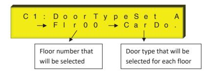
Also if all door types are the same type, "All" on the left side floor screen is selected, it is pressed ENTER button and door type is selected with second arrow on the right side and all floors door types are defined the same type.
