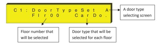
For selection, with lightening left arrow by pressing ENTER button, required floor is selected.
