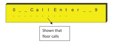
Dots on the screen indicate floor numbers in order. Floor that will be given call is selected with cursor and put "+" sign with "ENTER" on the floor number. More than one call, the other floors are selected the same.
